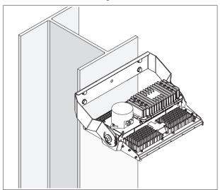
NOTE: XBLADE 480 can rotate 360°. Please be aware of the power cable's position with respect to the angle of the luminaire, avoid cable damage due to excessive bending. When using the locking / securing screws 1 screw per side will be sufficient however some angles allow for an additional screw if desired.
